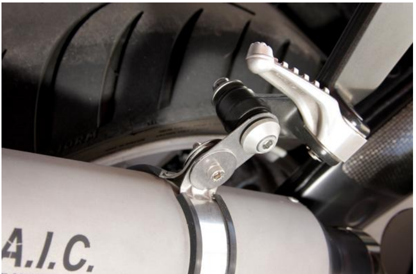
Figure 7: Installation of the Muffler Hanger Strap
