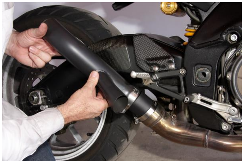
Figure 4: Installation of the Mid-Pipe
