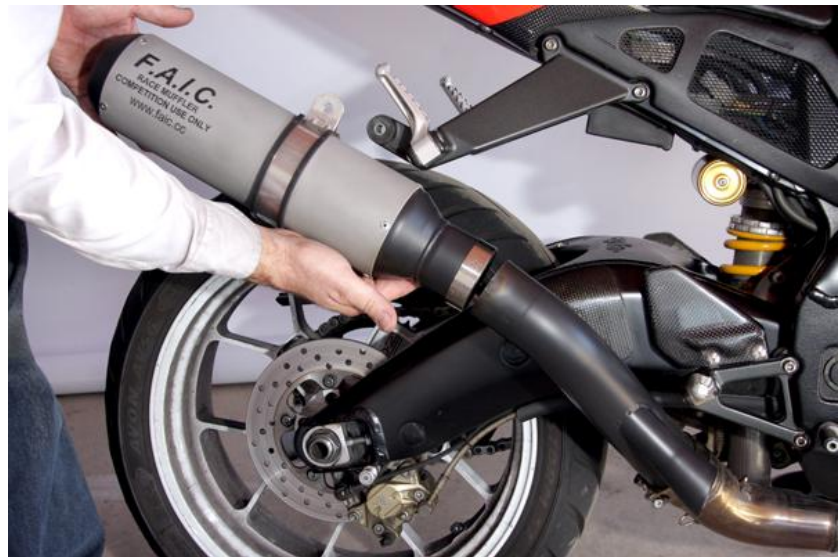
Figure 5: Installation of the Muffler
