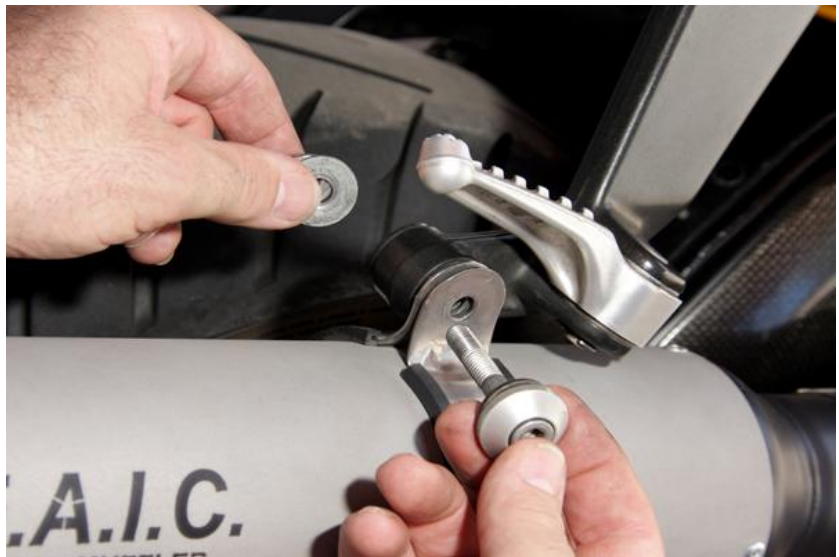
Figure 6: Installation of the Muffler Hanger
